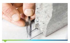
◆ Carbon prestressed concrete, reinforced with prestressed carbon fibers
